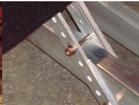
Standard ski-bunk kit allows significant bunk adjustment
